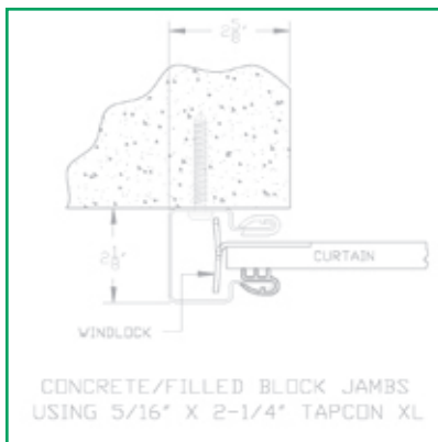
16 GA GUIDE MOUNTING DETAIL (for opening widths over 6'0" through 10'-0")
